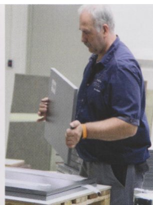
>at the left: these are the finished fronts after cutting. To cut the fronts, they need to be turned around. Apart from this fact the fronts are lying on the front side and the barcode is on top. On the right: quality control through an employee
