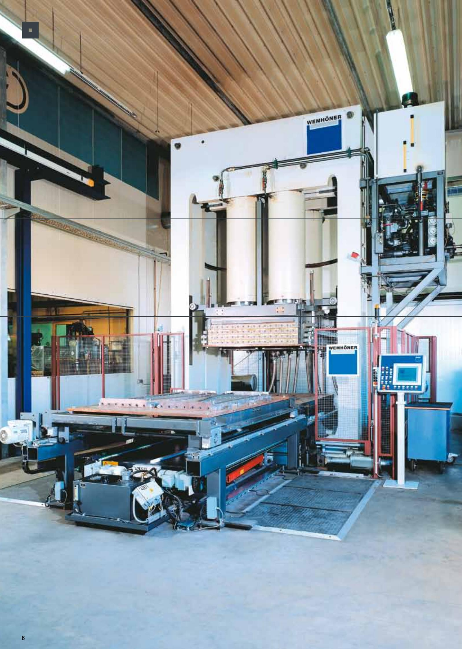
Wemhöner Moulding and Vulcanising Press Lines offer a wide range of applications to manufacturers of composite materials. Rubber-metal, Aramid or GRP composites are only some examples of custom-made products. The specific pressure of these lines are around 650 N/cm<sup>2</sup> and provide total press capacities of 24,000 kN.
