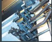
Wemhöner Multi-Daylight Throughfeed Presses can be installed on top of or next to one another. Infeed and outfeed is done fully automatically. The transport of workpieces within a press daylight is handled by linear guided foil belts. The press pistons positioned above the pressing plates ensure an even distribution of pressure from less than 10 N/cm² to more than 200 N/cm². Fluids such as thermal oil or hot-water heat-up the heating plates to a temperature of up to 130°C.
