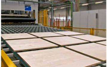
The Wemhöner Throughfeed Press Lines in single-daylight execution are ideal for the value adding process of covering wood based panels with veneer. They are mainly used for the production of materials for the door, panel and flooring industry. Both the entry level models and the fully automated systems can be equipped to provide the utmost flexibility for small to large series production.
